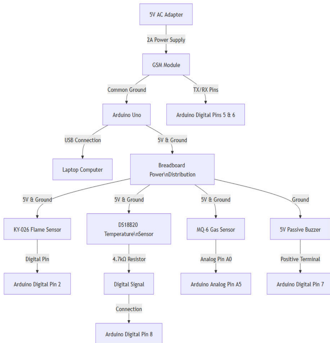
Figure 1. System architecture block diagram showing interconnections between Arduino Uno, flame sensor (Pin 2), temperature sensor (Pin 8 with 4.7k \Omega pull-up), gas sensor (A5), GSM module (separate 5V/2A supply), and buzzer (Pin 7).
